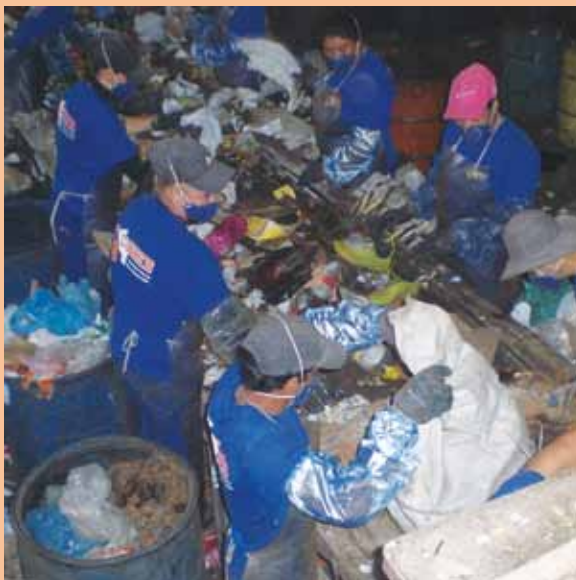
Photo 11: Manual sorting of dry recyclable materials from mixed waste: Use of PPE in sorting and conditioning (© Thilo Schmidt)
